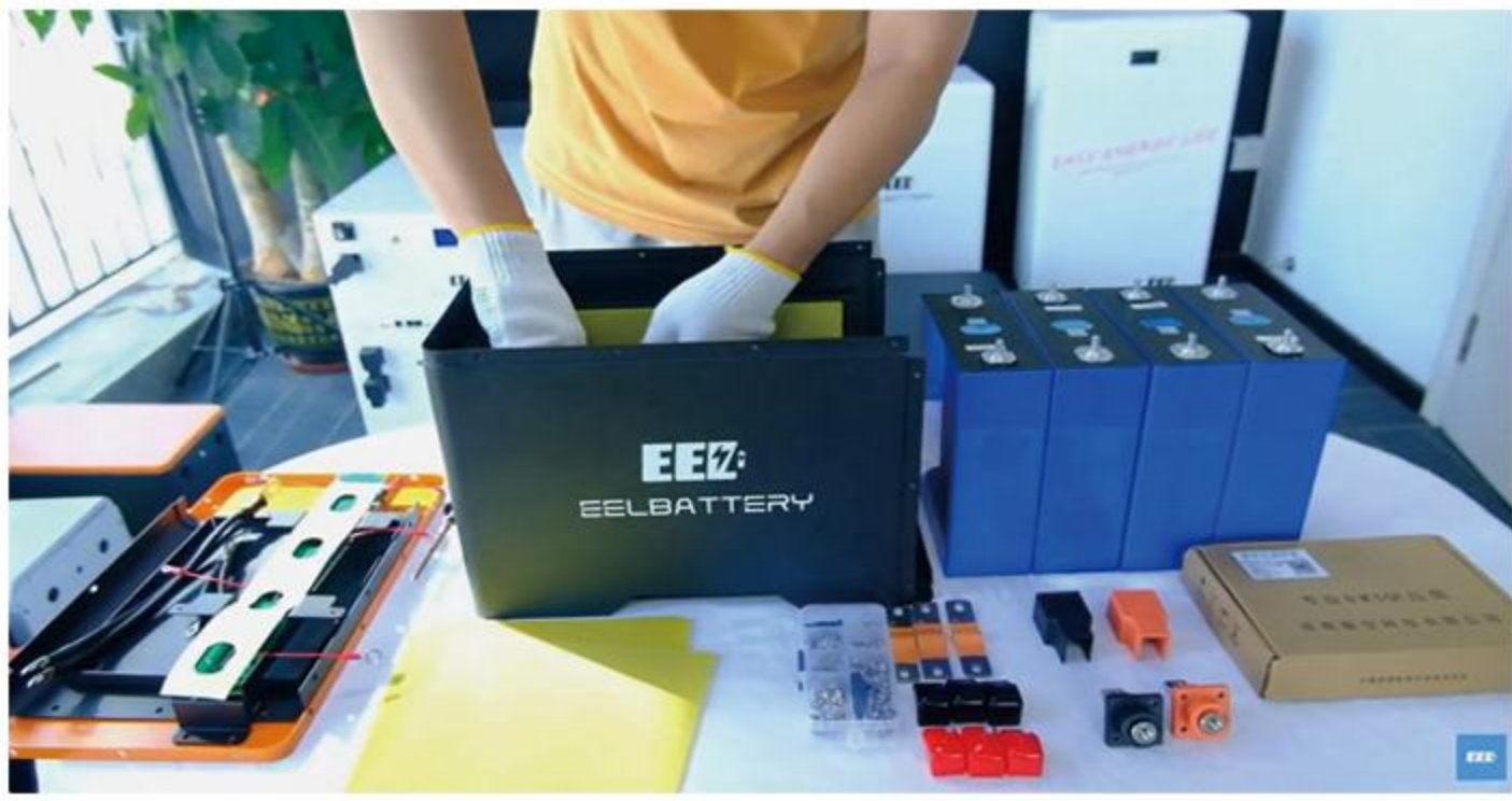
1. Paste epoxy sheets of corresponding sizes on the bottom and around the battery box.
