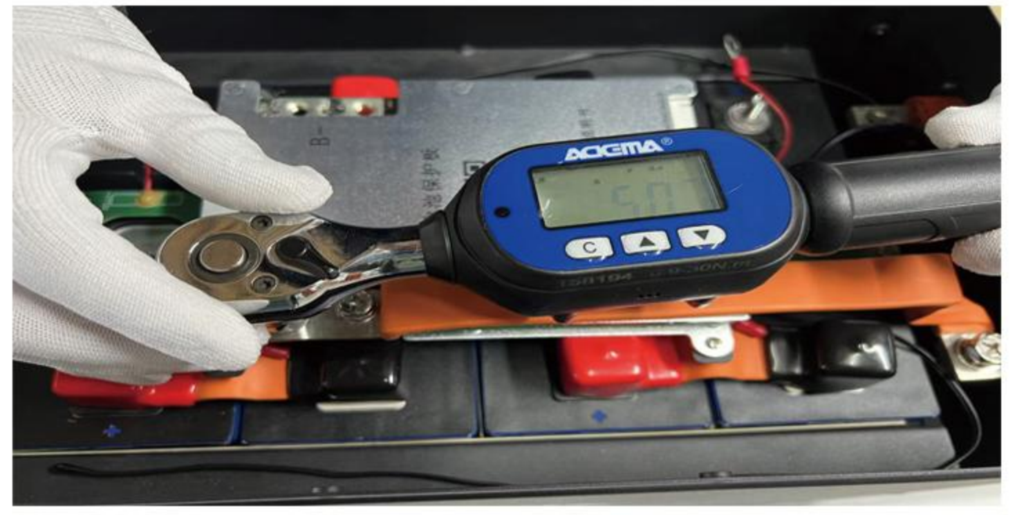
22. Tighten the screws with a torque of 5NM. Use M8 to connect the other end of the special busbar to the negative output terminal, and also tighten with a torque of 5NM.
