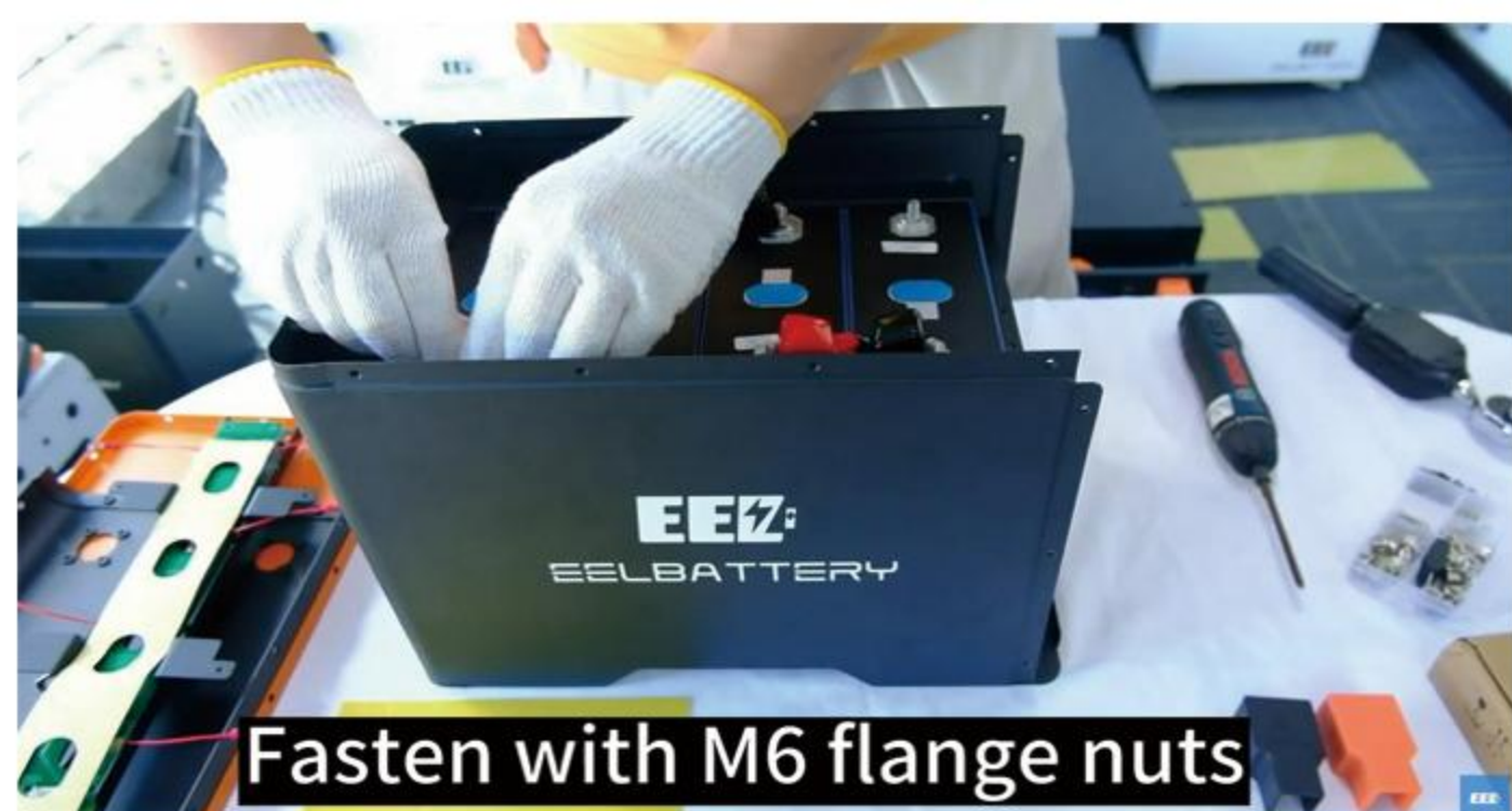
9. Lift one side of the insulating rubber cap by hand and screw the M6 nut onto the battery stud by hand.
