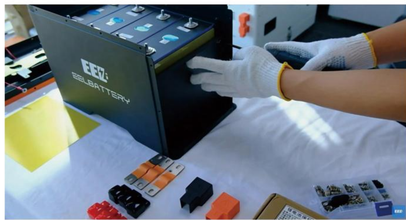
5. Use M5 screws to install the front baffle and tighten it with 5NM torque.
