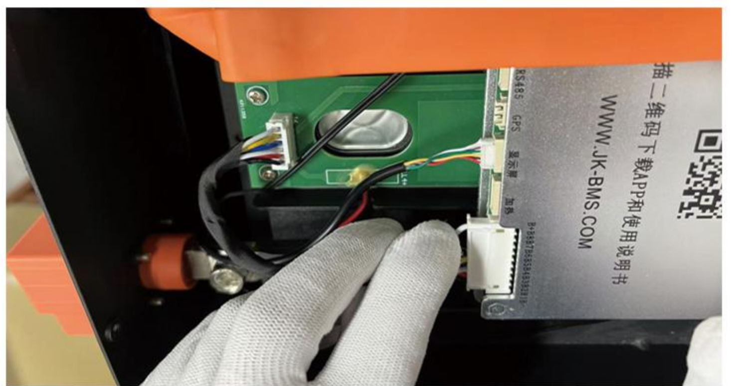
28. Connect the BMS sampling line to the corresponding port of BMS and plug in the switch line.
