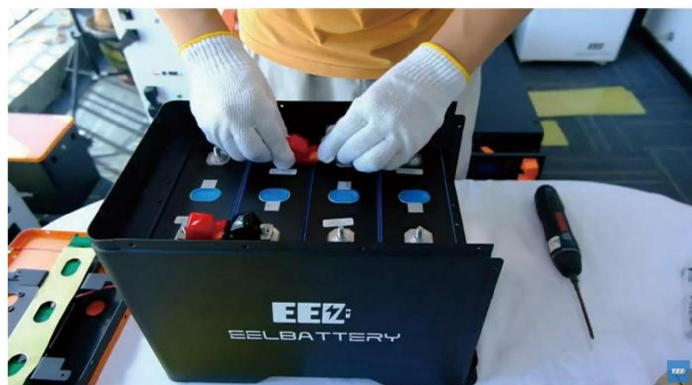
7. Place the busbars with rubber caps on the battery cells in order.
