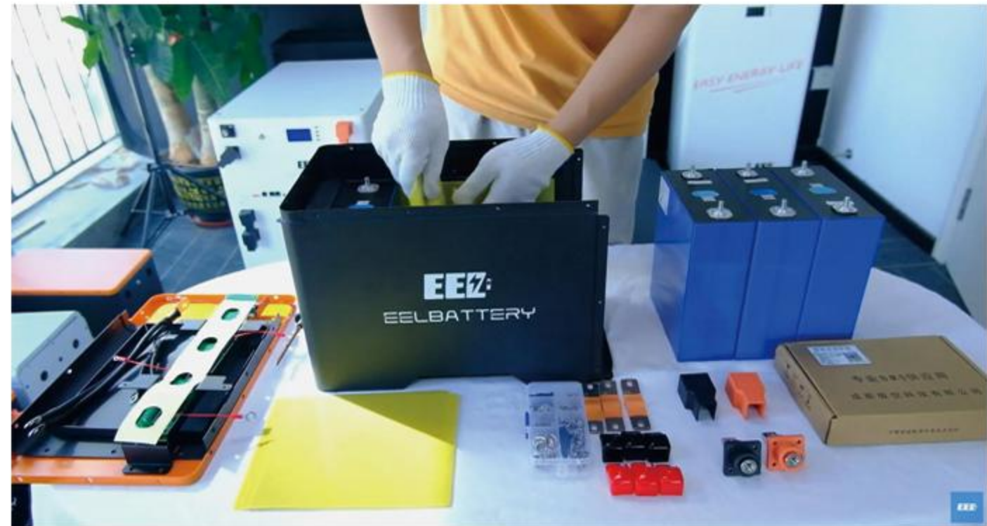
3. Place epoxy board and EVA sponge between the battery cells.
