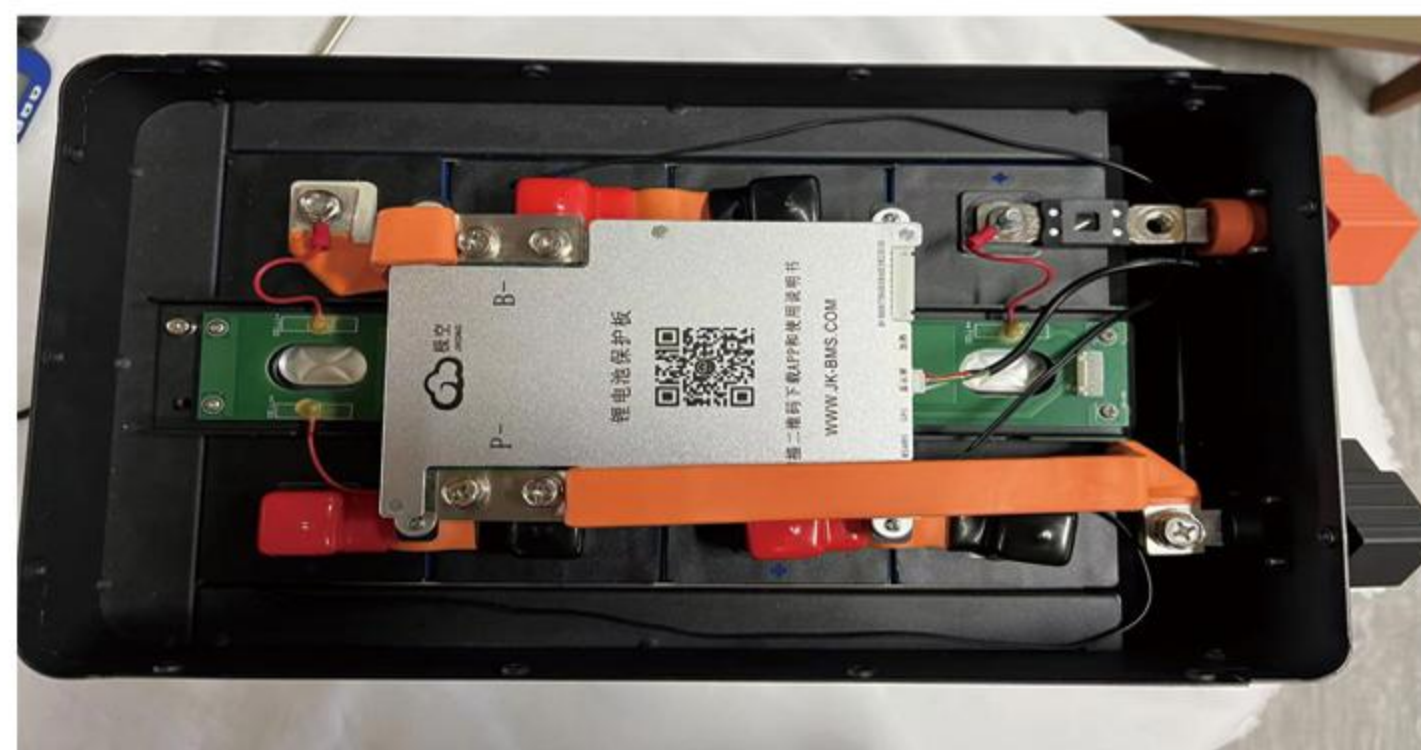
29. Plug the sensor plug into the BMS and place the temperature probe in a suitable place.
