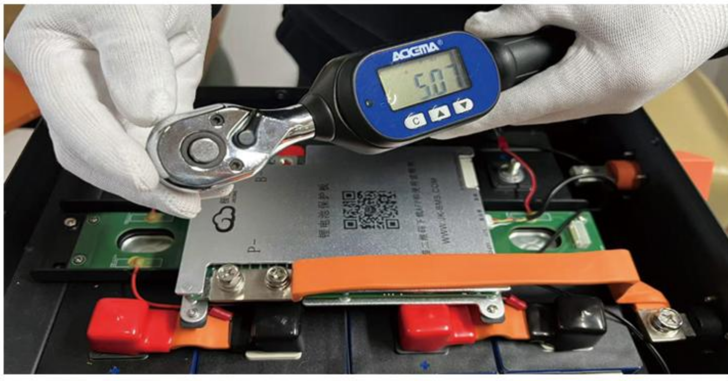
21. Adjust the torque wrench to 5NM
