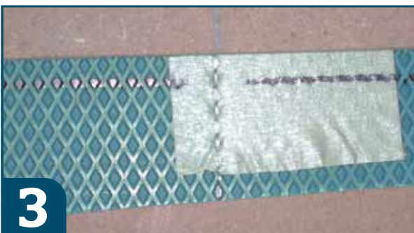
3 Determine correct direction that the texture should run. Draw a line on pattern board and align with pre-determined mark on FLEX-MOLD. Place pattern board on FLEX-MOLD and press down to adhere.
