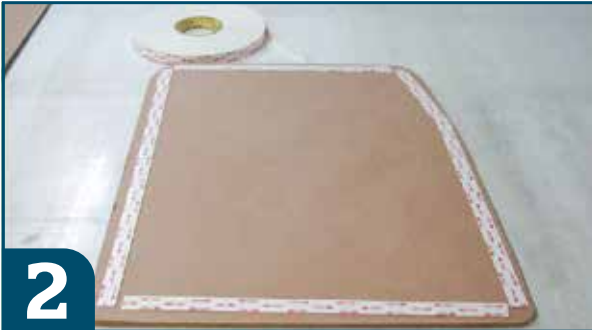
2 Apply double sided foam rubber tape around perimeter of pattern board.
