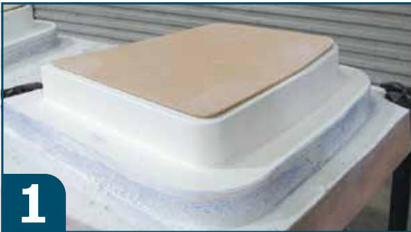
1 Cut a plywood or fiberboard pattern to exact size and shape required.
