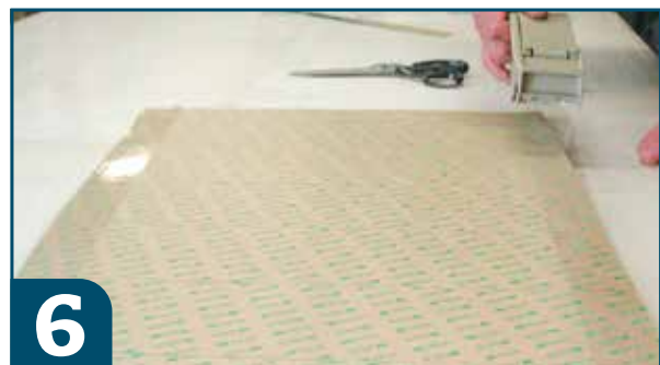
6 Apply clear packaging tape around border.
