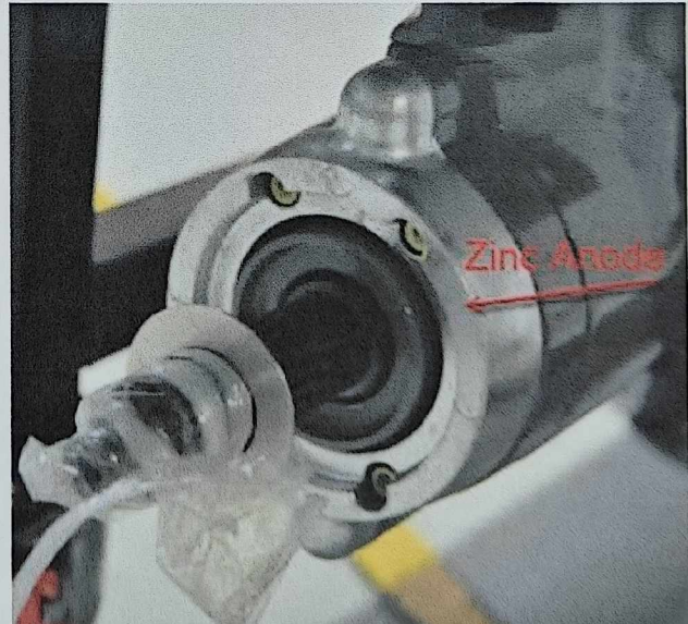
The three anodes should be checked with the boat is slipped and the saildrive oil is changed.
