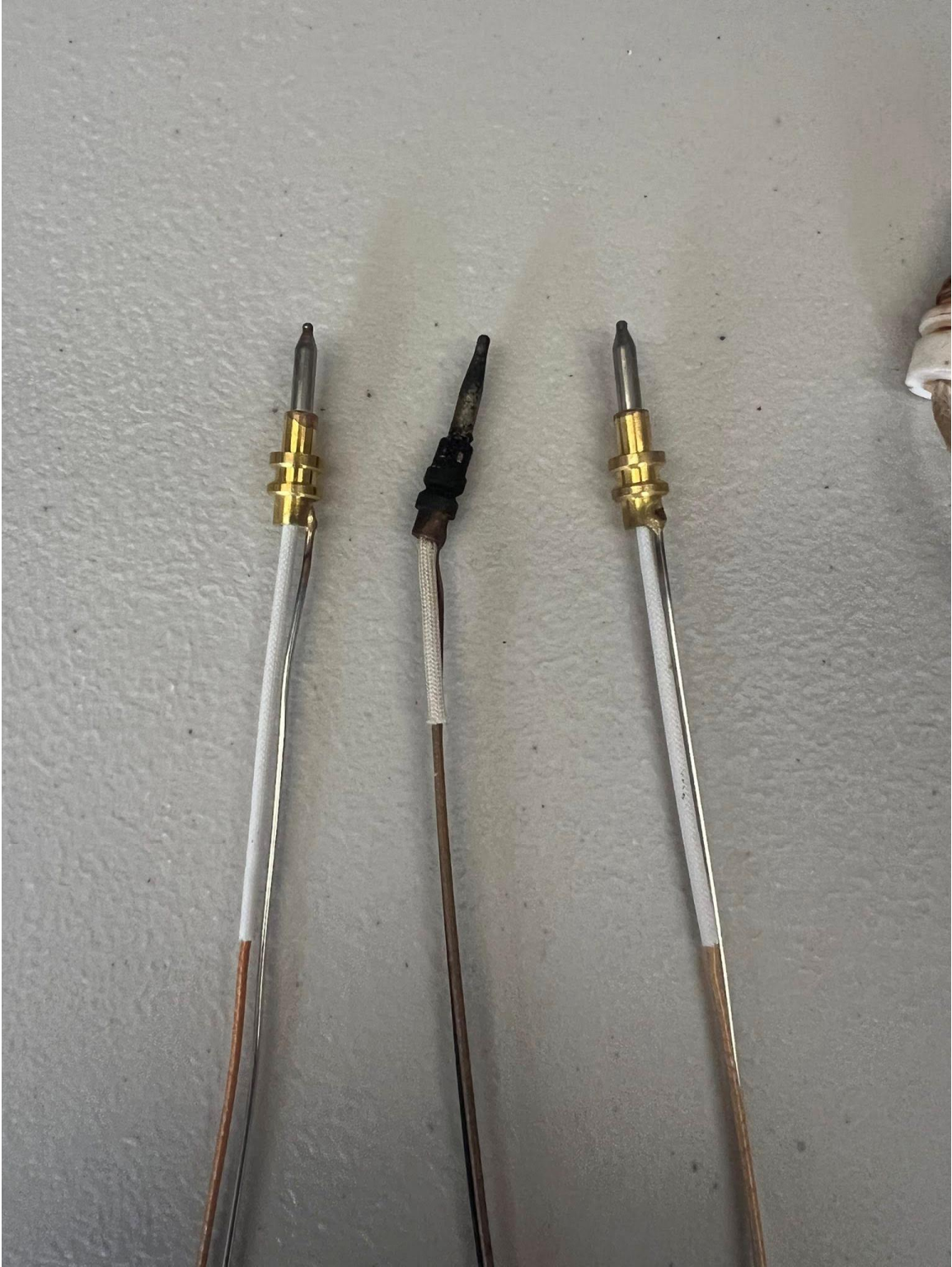
New thermocouples next to old one
