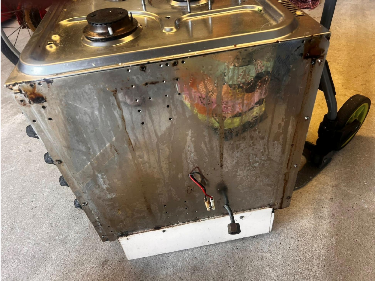
Control side panel, shows electrical and gas input fitting.
