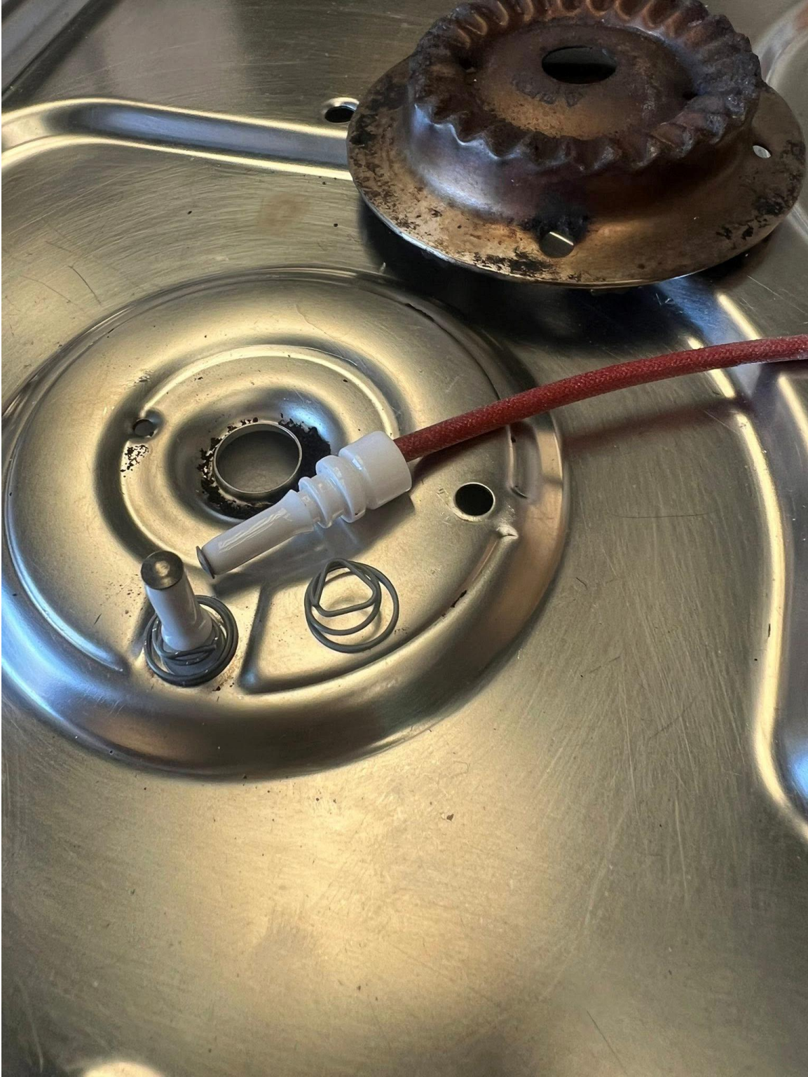
Pic of igniter in place note spring. Old one had a circlip to keep in place, this is better
